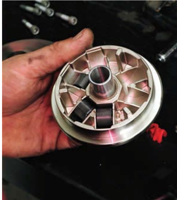
Inside the variator, you can see three of the rollers and, in the empty spaces, the ramps they have to climb to change gears.
